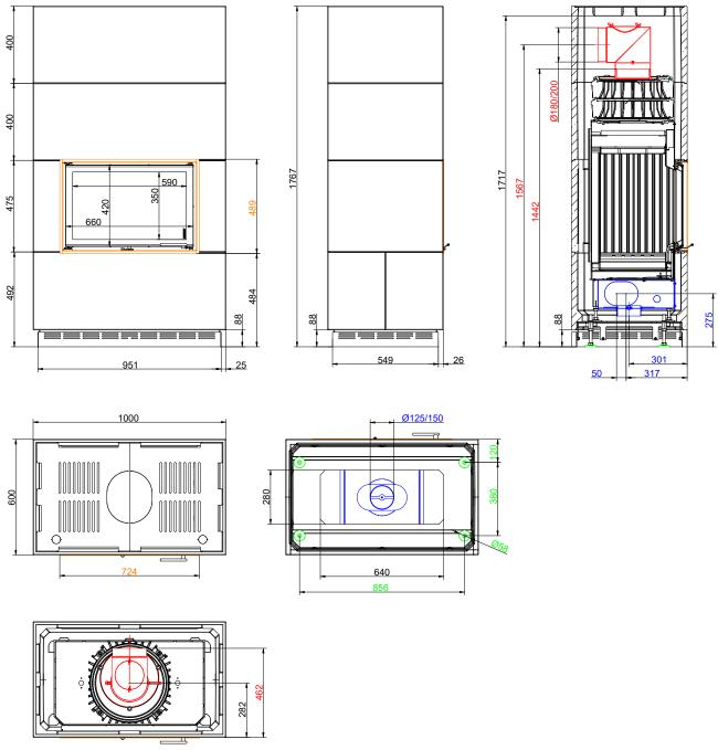
... with side opening door frame (orange), combustion air nozzle (blue), levelling feet (green)
